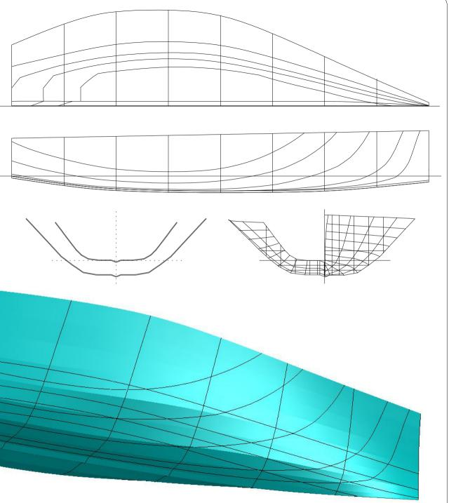
Maximum beam: 2090 mm Waterline beam: 1057 mm Hull draft: 155 mm LCB: 2377 mm
